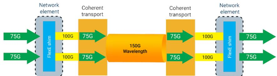
Figure 6. Sub-rating interop with coherent technologies
