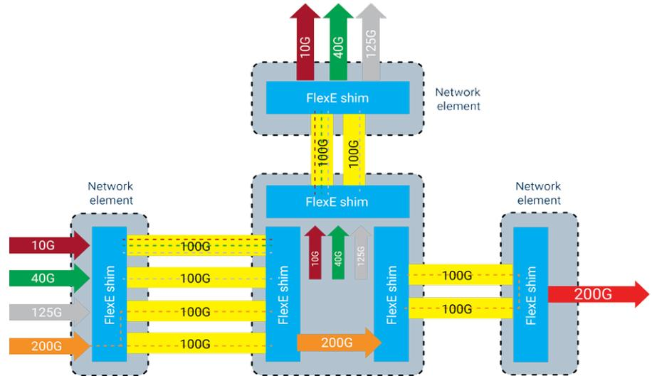
Figure 7. FlexE channelization example
