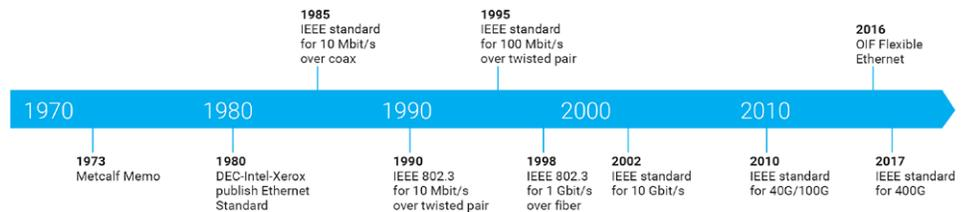
Figure 1. Introduction and evolution of Ethernet over time
