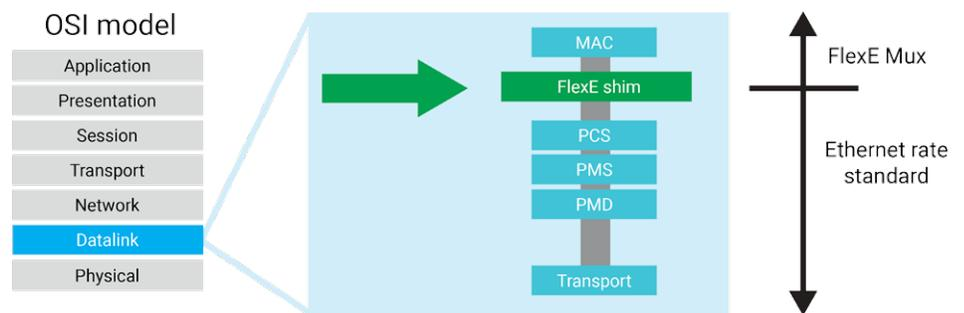
Figure 4. Characteristics of FlexE shim
