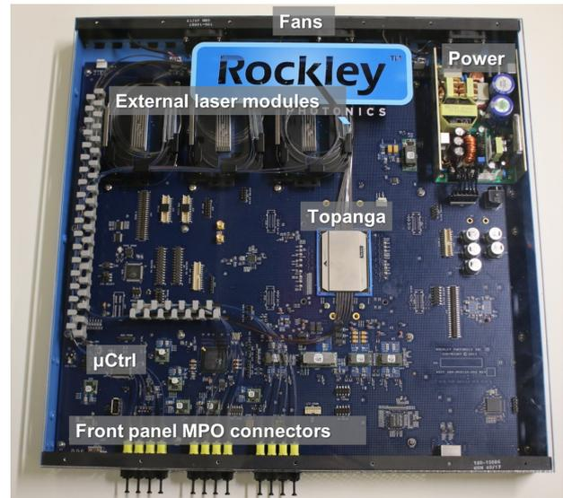
Figure 5: 1RU Ethernet switch box with 12x100GE ports. The *Topanga* device implements a Layer-3 switch ASIC along with parallel single-mode fiber optics for all ports. External laser modules supply the optical power. This switch consumes less than 3W per port, which is lower than the typical per-module power of a 100GE optical module alone, but includes all switching and routing functionality.
