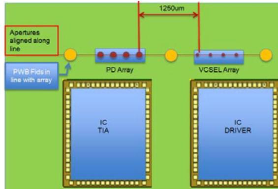
Figure 11: VCSEL/PD Array Assembly Example – General Layout
