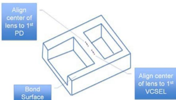
Figure 14: Plastic Molded Lens Example (Upside Down)
