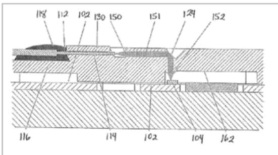
Figure 9: Integrated Plastic Molded Lens Cross Section
